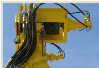
Hydraulic lifting and direction motors for the crab, independent for each function
